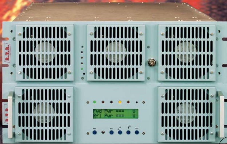
FM Mosfet Amplifier 87.5-108 MHz range
